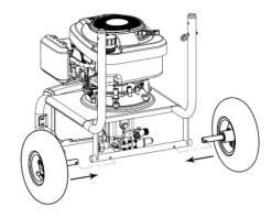
Attach the handle and main frame with knobs and bolts.
